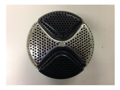
**Hazard:** The drain suction cover can become disengaged from the spa wall, posing an entrapment hazard to consumers.
