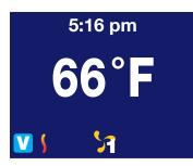
6. Press the SWIM WORKOUT button again to turn OFF the pump - the red **SWIM** icon on the LCD screen turns OFF.
