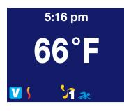
Press the SWIM button to turn the pump ON – the blue SWIM icon on the LCD screen turns ON.
