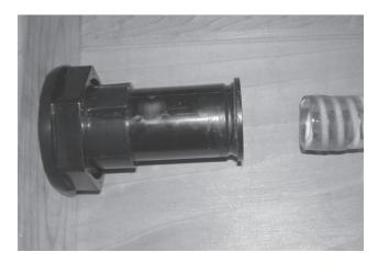
4. The spa drain is designed to be used with ¾" spa flex hosing. Cut the flex pipe long so that it can travel back and forth freely with spa drain internal then glue it into the back of the spa drain using the proper PVC sealant.
