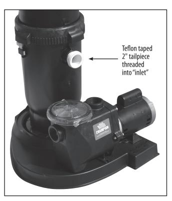
3. Place filter inside base. Wrap 3 or 4 turns of Teflon tape on 2" tailpiece and thread into "inlet" in filter. **DO NOT** insert snap pins through (secure) motor base until Step 3 is complete.
