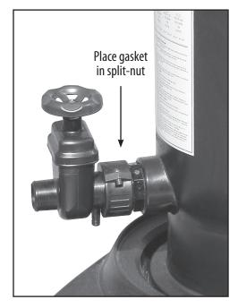
6. Place the other 1  $\frac{1}{2}$ " gasket in gate valve split-nut and thread onto 2"x 1  $\frac{1}{2}$ " MPT union fitting.
