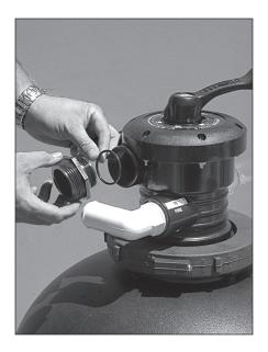
7. Take O-ring and put over small side threads on 1 ½" buttress x MPT fitting. Thread onto pump outlet on multi-port valve (top port).
