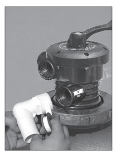
**6.** Apply Teflon tape to 90° smooth hose adapter threads (4 wraps) and and thread into the bottom of the multi-port (to pool).
