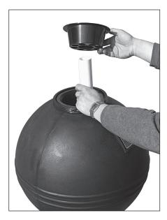
2. Place sand filter guide in filter over stand pipe. Add approximately 3 inches of water before adding sand. Add required #20 grade silica sand (see sand chart on back page). Remove sand filter guide and save.
