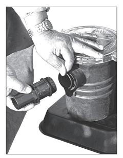
**12.** Put 0-ring over threads on 1 ½" smooth straight hose adapter and thread into front of pump basket.
