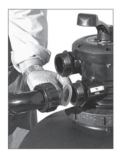
Put 1 ½" gasket into return sweep assembly and install onto pool outlet port.
