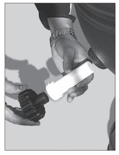
16. To remove drain screen, remove drain screen cap/wrench and insert the wrench end into drain screen opening and unscrew. When reinserting drain screen DO NOT OVER TIGHTEN (be sure 0-ring is inside of drain cap). Screw on drain screen cap/wrench. DO NOT OVER TIGHTEN.
