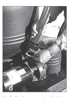
11. Put 2" gasket into nut on hose labeled "TO VALVE PUMP PORT."
