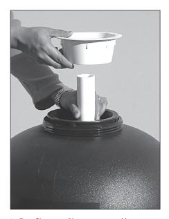
Turn filter over. Place next to pool between skimmer and return opening on pool. Place sand filter guide in filter over stand pipe.
