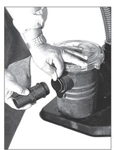
**11**. Put 0-ring over threads on 1 ½" smooth straight hose adapter and thread into front of pump basket.
