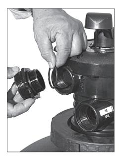
7. Take 0-ring and put over small side threads on 1 ½" buttress x MPT fitting. Thread into pool outlet on valve. Repeat for pump outlet on valve.
