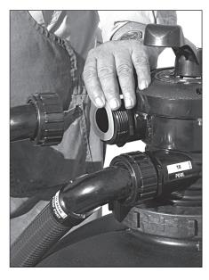
Take pump to filter hose assembly and put 1½" gasket into nut on smaller end with sweep 90°. Thread onto pump outlet port.
