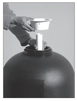
2. Turn filter over. Place next to pool between skimmer and return opening on pool. Place sand filter guide in filter over stand pipe. Fill tank approximately ¾ full of water before adding sand. Add required #20 grade silica sand (see sand chart on back page). Remove sand fill guide and save.
