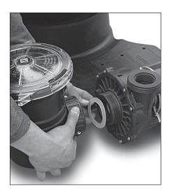
6. Install trap base to pump by removing gasket from inside trap. Remove clear trap lid, and place gasket in trap nut. Thread onto pump. DO NOT OVER TIGHTEN. Place pump with trap onto pump base. Remember to replace trap lid.
