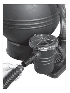
14. Install 6 ft. corrugated hoses by loosening hose clamps and sliding over hose ends. Install hose onto pump basket hose fitting by pushing on and tightening clamp. Install other end of hose onto skimmer and tighten clamp.
