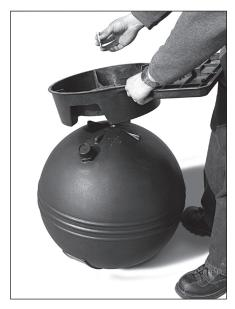
Attach filter base to filter body by turning body upside down. Align drain on filter with clearance slot on base. Slip washer over bolt and thread bolt into filter body. DO NOT OVER TIGHTEN.
