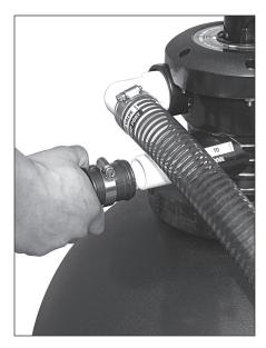
15. Install hose onto smooth hose adapter in valve by loosening hose clamp and sliding over adapter end. Install other end onto return fitting of pool and tighten clamps.
