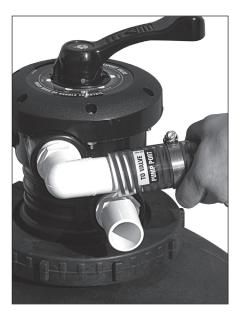
**10.** Install pump hose labeled "TO VALVE PUMP PORT" by sliding hose with metal clamp over smooth 90° adapter and tighten clamp.
