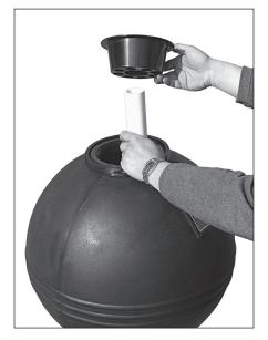
Turn filter over. Place next to pool between skimmer and return opening on pool. Place sand filter guide in filter over stand pipe. Fill tank approximately ¾ full of water before adding sand. Add required #20 grade silica sand (see sand chart on back page). Remove sand fill guide and save.
