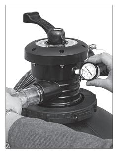
**13.** Apply Teflon tape to threads of pressure gauge (4 wraps is ideal) and thread into valve. Install waste adapter by pushing 0-ring over threads of clear adapter and threading into waste port.
