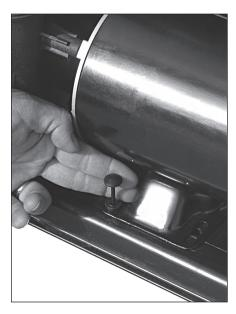
7. Install anchors into slots of pump, and then into the holes in the pump base. Be sure to place pump on base where "Mounting Holes for Sand Filter" is shown. Push pins into anchors to secure.
