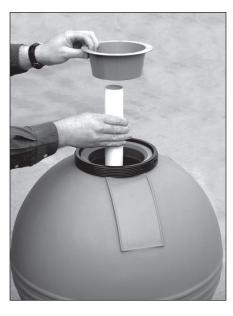
Turn filter over and place sand fill guide in filter over stand pipe. Fill with water before adding sand. Add required #20 grade silica sand (see sand chart). Remove sand fill guide and save.
