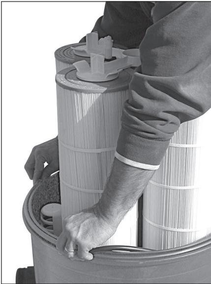
1. Start at back (opposite side from fittings), place O-Ring around lip of filter and draw it toward you putting O-Ring between thumb and forefinger.
