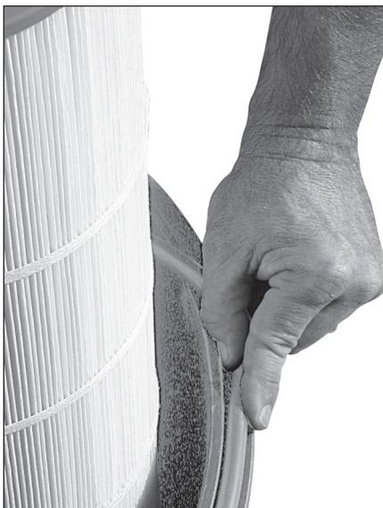
3. Continue drawing O-Ring toward you, keeping thumb and forefinger between O-Ring and filter lip.
