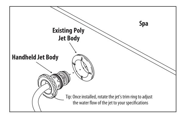
To install the handheld jet, unscrew an existing Waterway poly jet (turn counterclockwise). The existing jet may require a jet wrench for removal, available from your local spa retailer.
