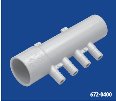
MANIFOLD 1" S x 1" SPG x (4) 3/8" RB
